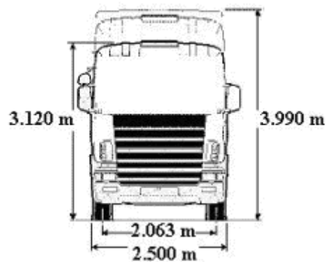
Fig.6 – Dimensions of a frontal surface of a typical transport vehicle.
