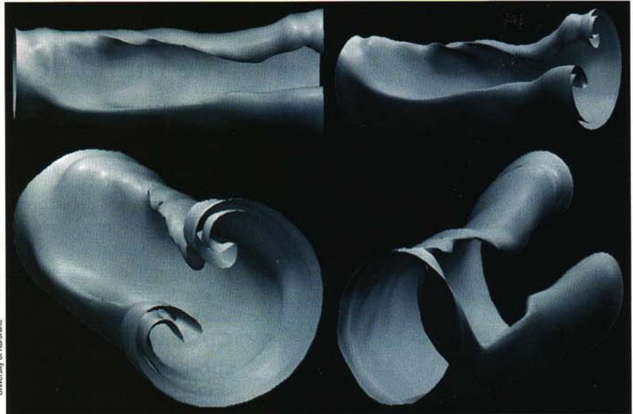
Tomography: Bodo Ruck and colleagues at the University of Karlsruhe synchronize the scans of a laser sheet with a video camera running at rates of up to 200 frames per second to produce three-dimensional tomographic impressions of phenomena in fast liquid flows. The images combine frames of approximately 20 light sheets to illustrate the development of a 23 mm long free jet as it flows from left to right and expands from 3 to 9 mm under the influence of a crossflow.
