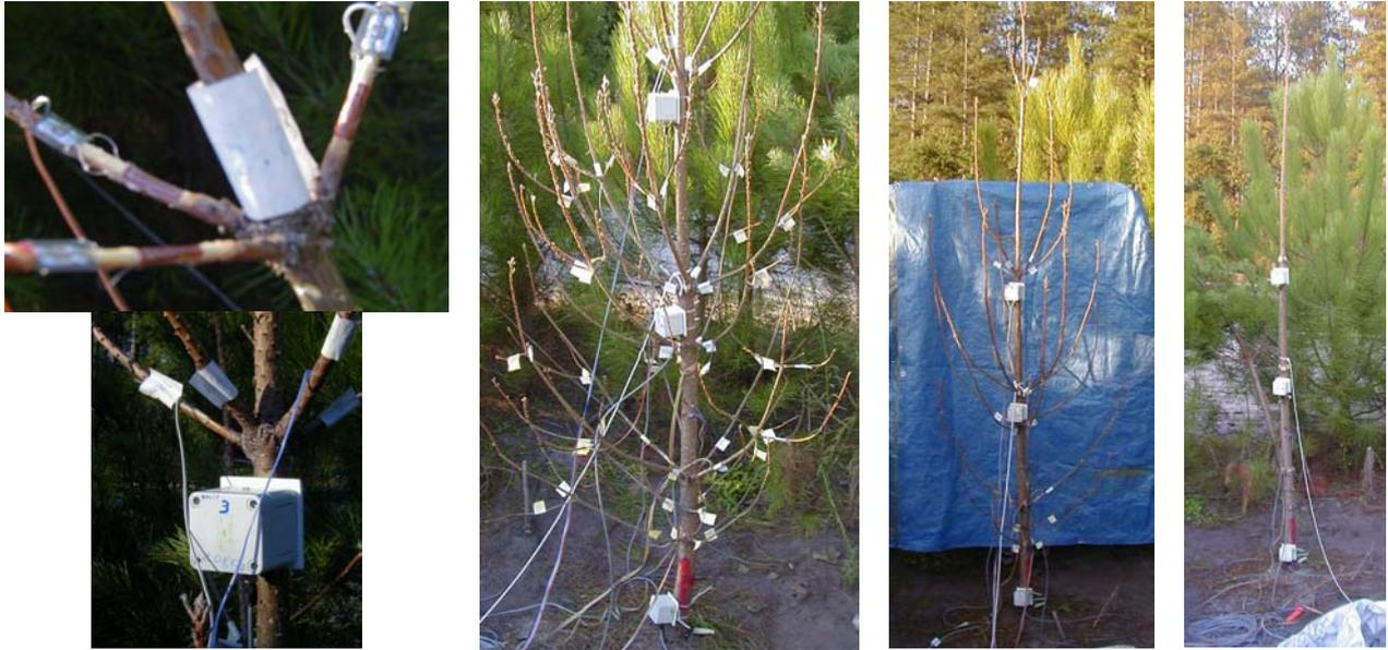
Figure 1: The tree (T1) through the different phases of pruning. 3 strain gauges were glued on 3<sup>rd</sup> order axes in a/, an inclinometer attached on the stem in b/. The first phase of pruning consisted in removing the needles (c/), then in removing the 3<sup>rd</sup> order axes (d/) and finally in removing the 2<sup>nd</sup> order axes so that stem (1<sup>st</sup> order axis) alone was left.
