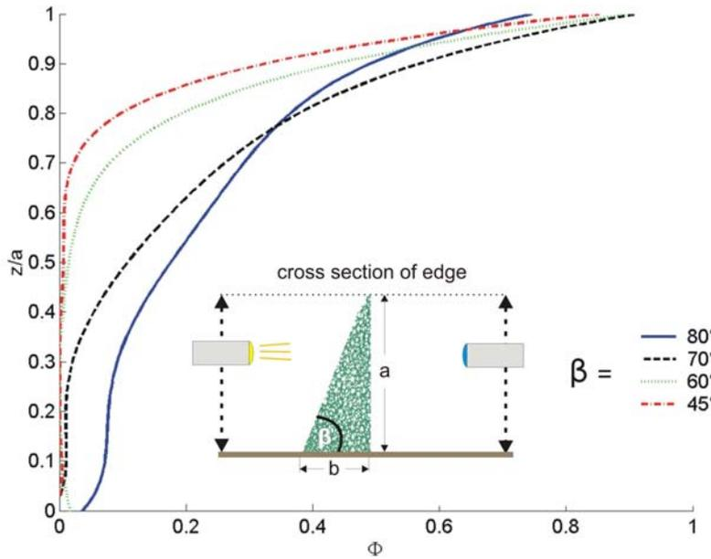
Figure 4: . Vertical profiles for optical porosity  $\Phi$  of edge models with varied angle, as determined photographically. Note: the 80° curve theoretically should not cross the other. Deviation is due to difficulties in slicing the material at sharp angles.
