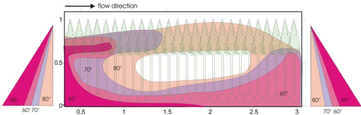
Figure 6. Zone of positive pressure coefficients inside the forest (coloured area) as a function of forest edge angle ( $45^\circ$  to  $80^\circ$ , see tab. 1 for details); smoothed data.
