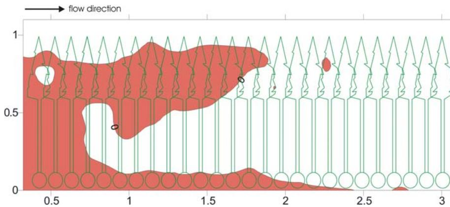
Figure 5. Zone of positive pressure coefficients  $c_{ps}$  in the edge-near region (coloured area); model forest with free airflow through the trunk space
