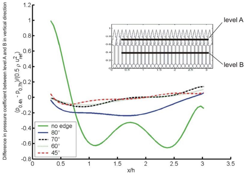
Figure 10. Pressure difference between trunk space (0.4h) and canopy (0.7h).
