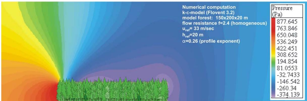
Fig. 8: Numerical computation of the pressure field around a small forest stand, 90°-edge
