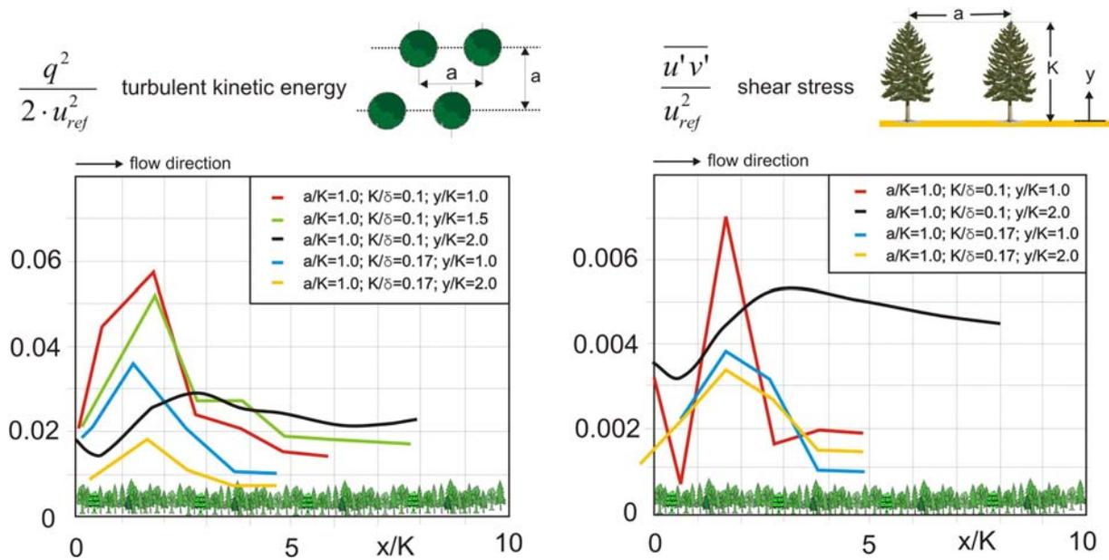
Fig. 1: Streamwise development of turbulent kinetic energy and shear stress after the forest edge at different heights above treetop level (Ruck & Adams, 1991)
