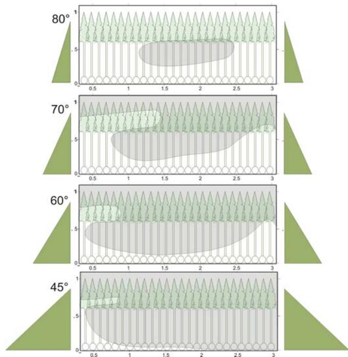
Fig.7: Zones of negative pressure coefficients inside the forest (shaded area) as a function of forest edge angle
