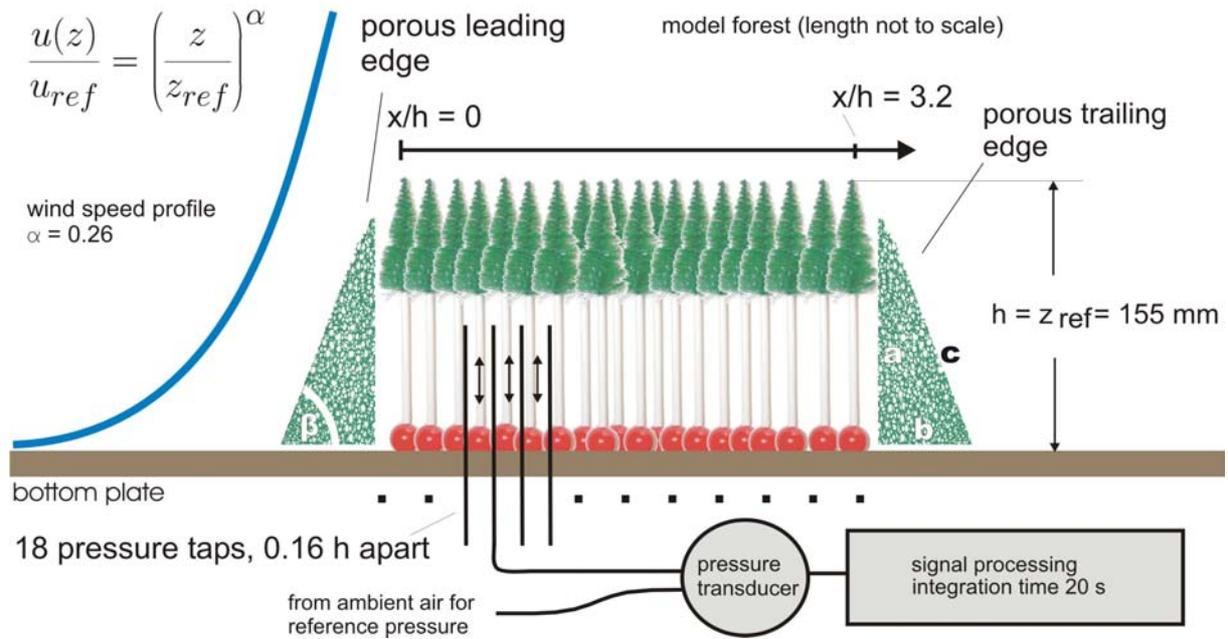
Figure 3. Experimental setup inside the wind tunnel with model forest, variable leading and trailing edges and measuring equipment.
