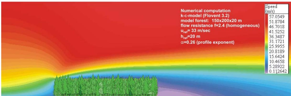
Fig. 9: Numerical computation of the velocity field around a small forest stand, 90°-edge
