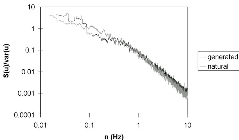
Fig. 1: Streamwise velocity spectra measure above a crop in natural and generated conditions.
