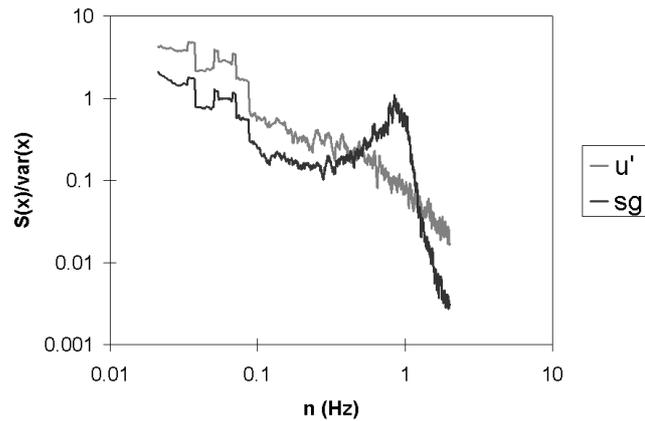
Fig.3 Displacement (sg) and velocity ( $u'$ ) spectra corresponding to a single stem.
