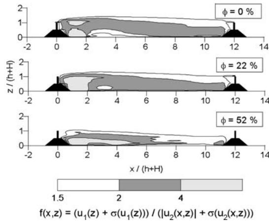
Figure 11. Contour lines of the pedestrian comfort parameter  $f$  as a function of porosity  $\phi$  at a distance between windbreaks  $a' = 12$ .
