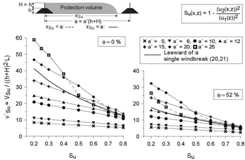
Figure 8. Dimensionless protection volume  $v'_{Su}$  as a function of protection parameter  $S_u$  with varying distance between windbreaks  $a'$  for two different porosities  $\phi$ .
