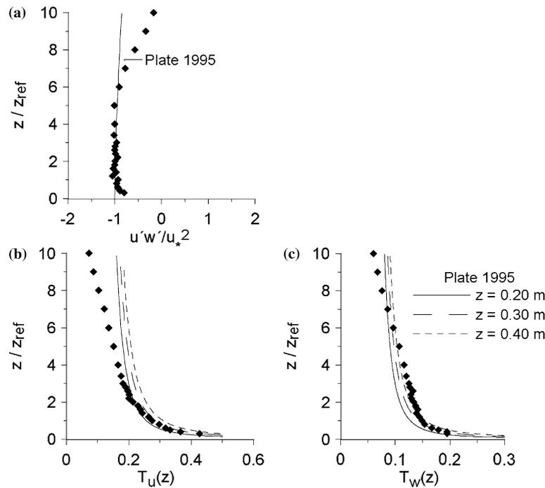
Figure 4. Simulated atmospheric boundary layer: (a) reynolds stress, (b) turbulence intensity in longitudinal direction, (c) turbulence intensity in vertical direction.
