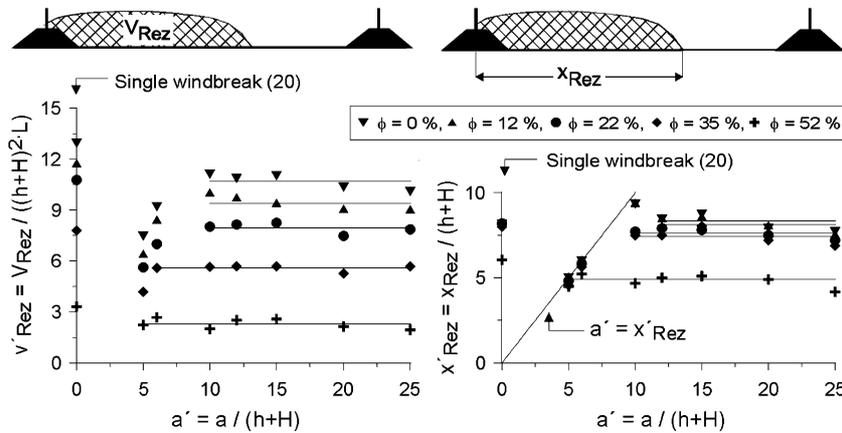
Figure 16. Dimensionless recirculation volume  $v'_{Rez}$  and reattachment length  $x'_{Rez}$  as a function of porosity  $\phi$  and distance between windbreaks  $a'$ .
