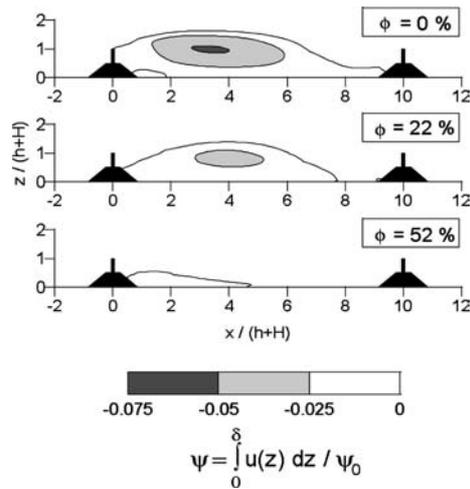
Figure 15. Recirculation zones as a function of porosity  $\phi$  at distance between windbreaks  $a' = 10$ .
