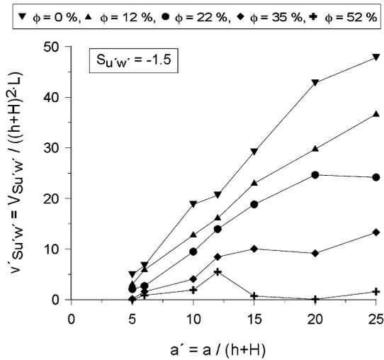
Figure 14. Dimensionless protection volume  $v'_{Su'w'}$  as a function of distance between windbreaks  $a'$  with varying porosities  $\phi$  for protection parameter  $S_{u'w'} = -1.5$ .
