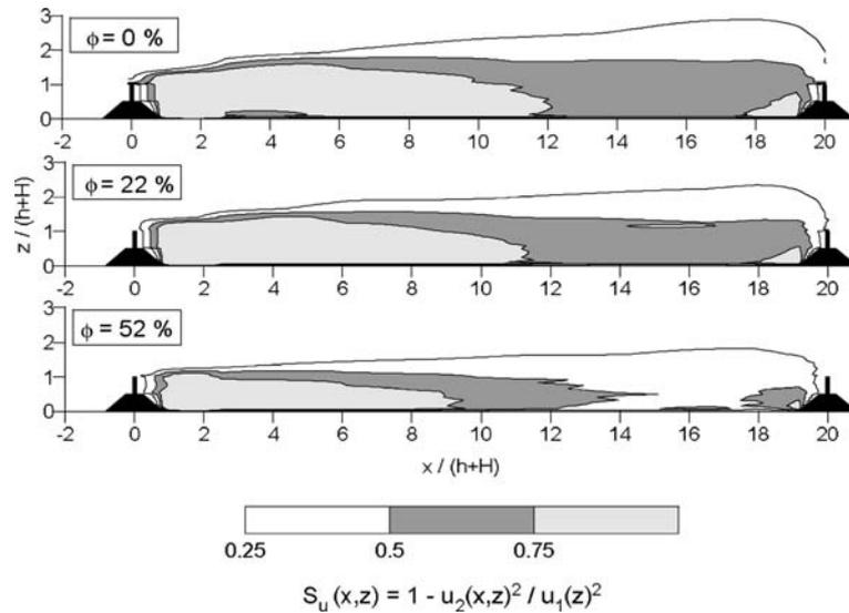
Figure 7. Contour lines of the protection parameter  $S_u$  as a function of porosity  $\phi$  at a distance between windbreaks  $a' = 20$ .
