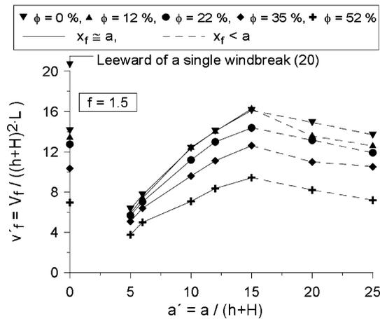
Figure 12. Dimensionless protection volume  $v'_f$  as a function of distance between windbreaks  $a'$  with varying porosities  $\phi$  for pedestrian comfort parameter  $f = 1.5$ .
