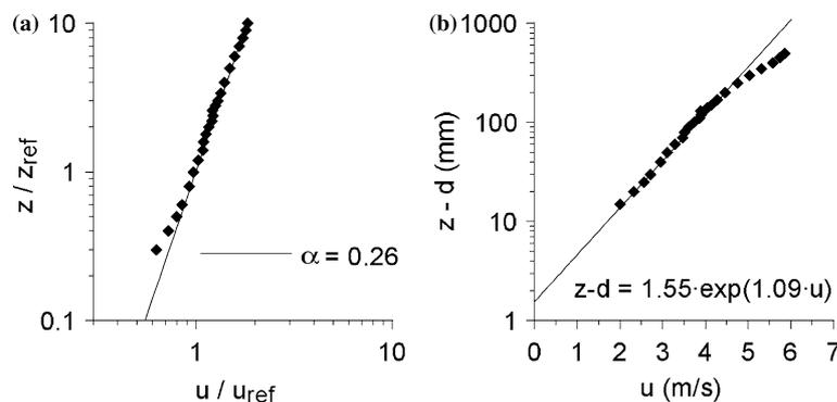
Figure 3. Simulated atmospheric boundary layer: mean longitudinal velocity (a) Power Law, (b) Law-of-the-wall.
