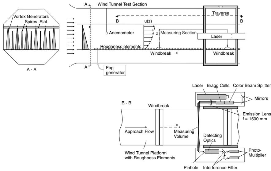
Figure 1. Sketch of the wind tunnel test section and the 2D-LDA-System.
