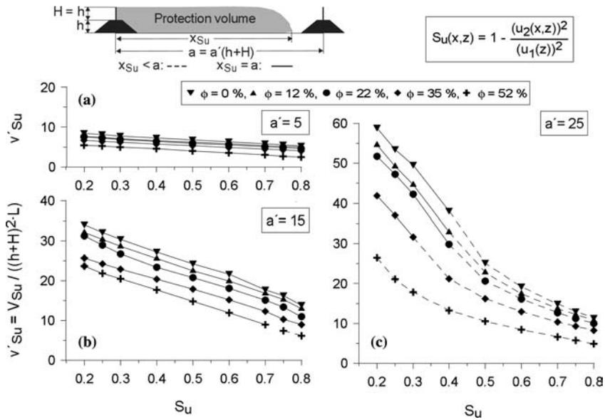
Figure 9. Dimensionless protection volume  $v'_{Su}$  as a function of the protection parameter  $S_u$  with varying porosity  $\phi$  for different distances between windbreaks  $a'$ .
