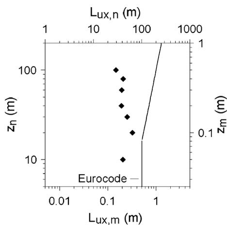
Figure 5. Simulated atmospheric boundary layer: integral length scale.
