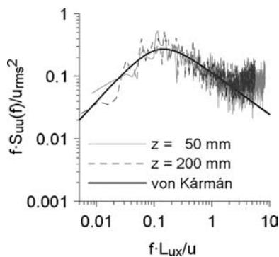
Figure 6. Simulated atmospheric boundary layer: spectral density function of the longitudinal velocity component.
