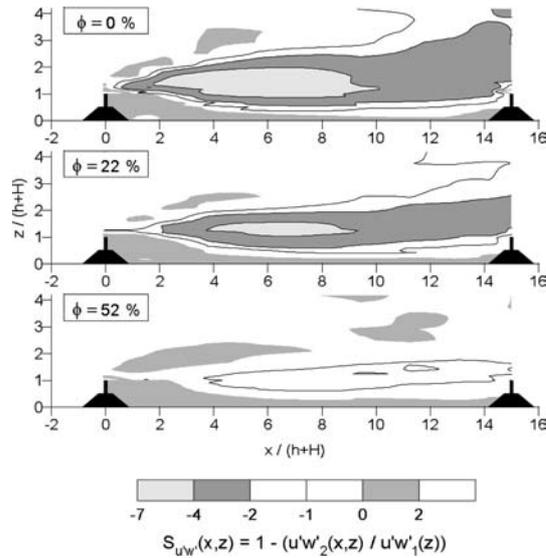
Figure 13. Contour lines of the protection parameter  $S_{u'w'}$  as a function of porosity  $\phi$  at a distance between windbreaks  $a' = 15$ .
