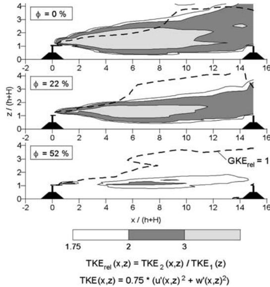
Figure 17. Contour lines of the relative turbulent kinetic energy  $TKE_{rel}$  as a function of porosity  $\phi$  at distance between windbreaks  $a' = 15$ . The dashed line plots the relative overall kinetic energy  $GKE_{rel} = 1$ . For regions under this line apply  $GKE_{rel} < 1$ , for regions above  $GKE_{rel} > 1$ .
