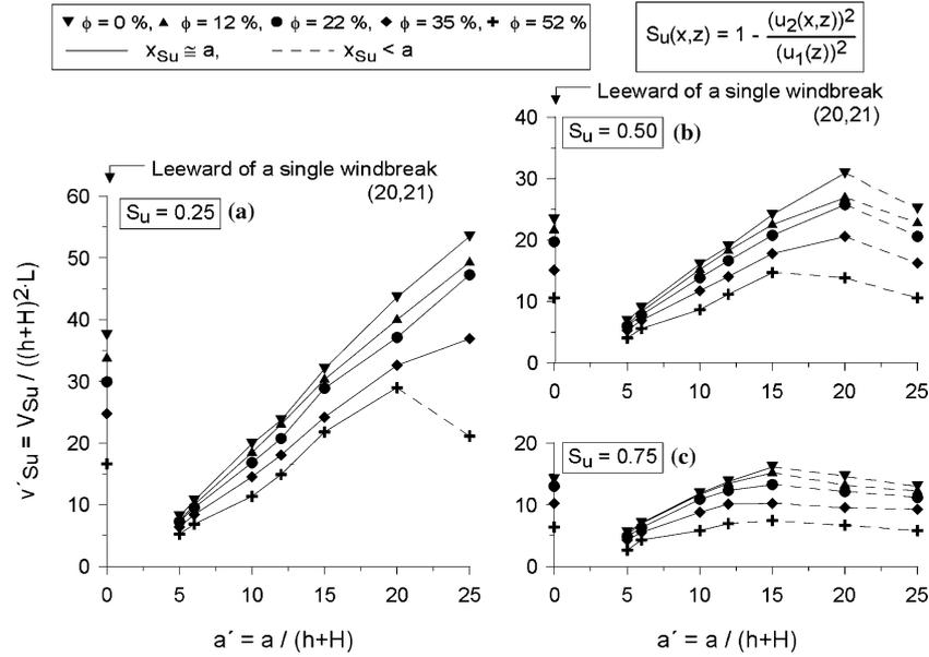
Figure 10. Dimensionless protection volume  $v'_{Su}$  as a function of distance between windbreaks  $a'$  with varying porosities  $\phi$  for different protection parameters  $S_u$ .
