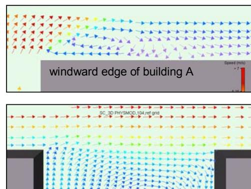
Figure 12. Vector plots of mean flow at roof level at  $y/H = 0.5$  for refined grid case
