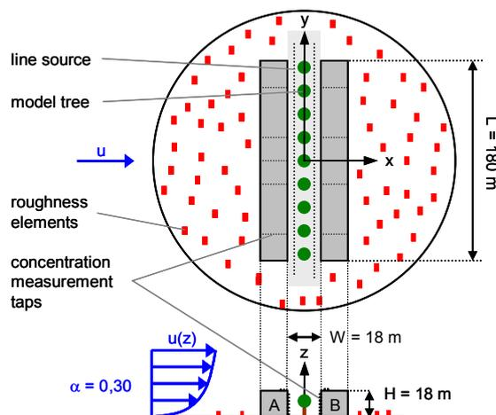
Figure 1. Model setup of street canyon (scale 1:150)
