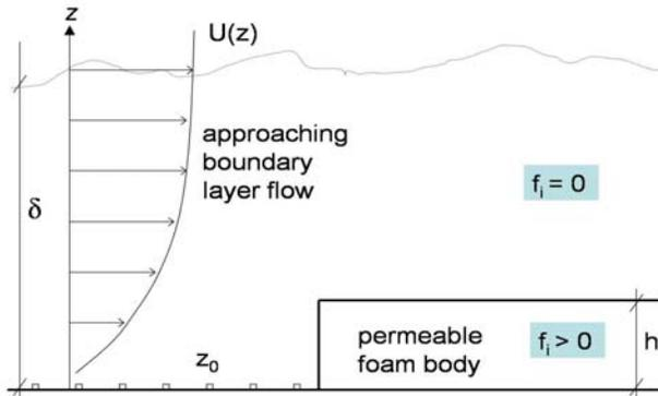
Figure 1. Experimental setup ( $f_i$ : additional body force in momentum equation, see eq. 1).
