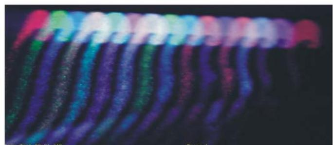
Fig. 6: Flow outlines or particle trajectories can intersect in the direction of detection. The detected outlines or trajectories may show defects, which can be repaired by image processing techniques.
