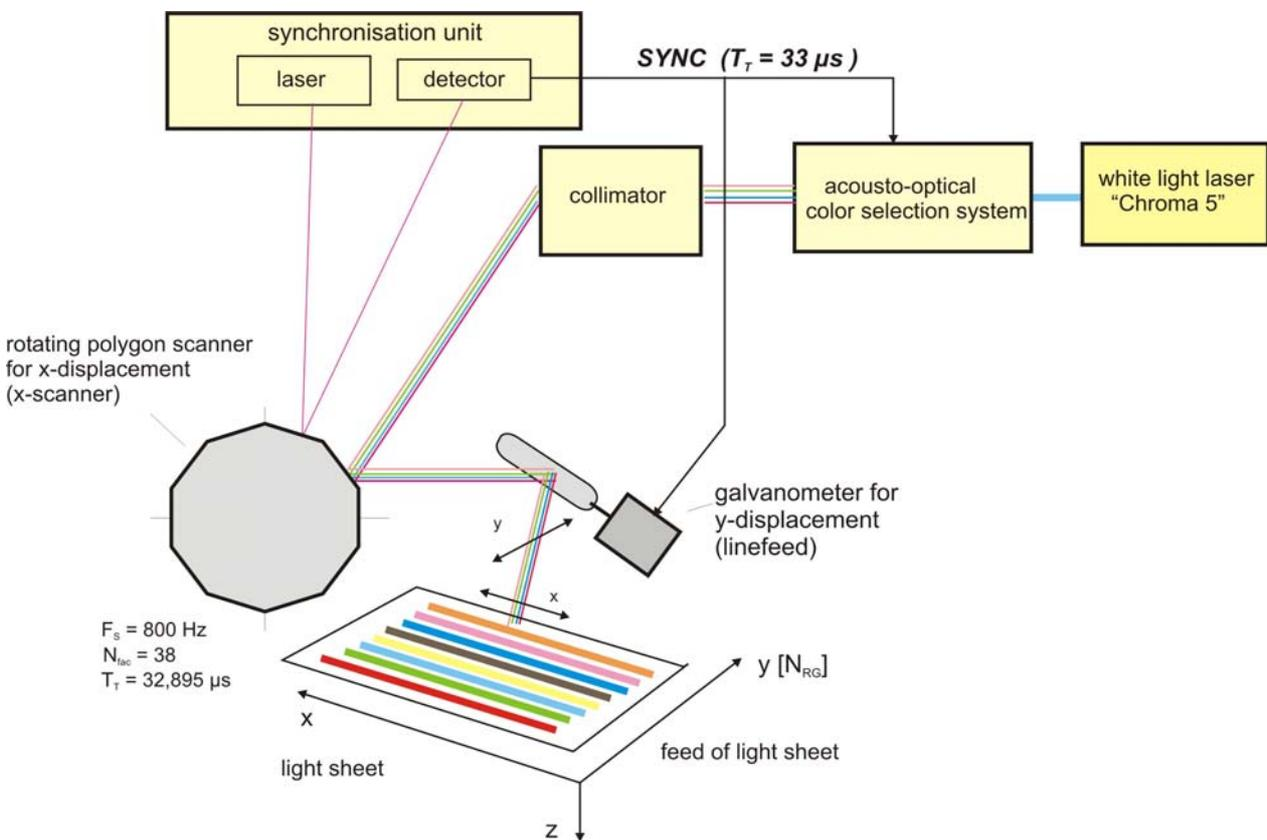
Fig. 2: Generation of differently colored laser light sheets
