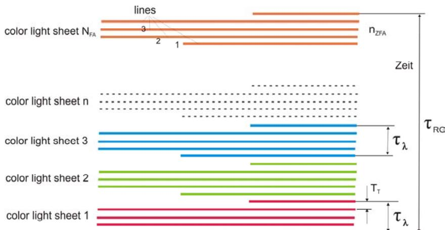
Fig. 3: Generating 'thick' colored light sheets by several lines of the same color
