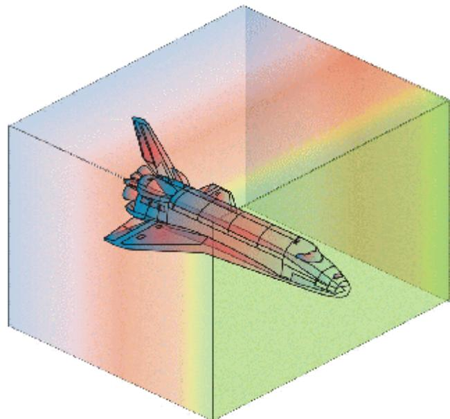
Fig. 1: Simultaneous illumination of a flow volume with colored light according to the natural light spectrum
