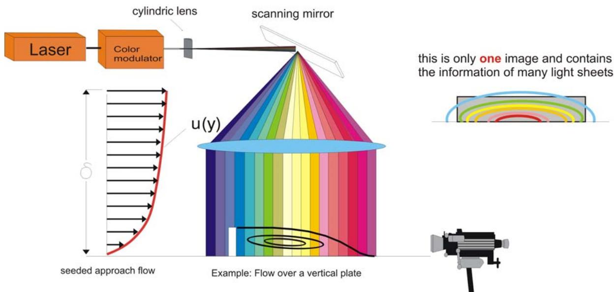
Fig. 4: Application of color-coded tomography for bluff body investigations
